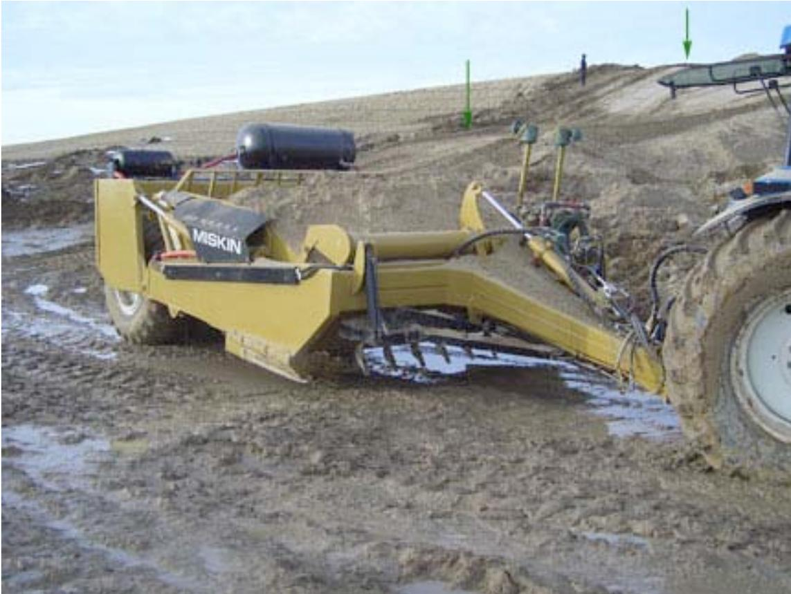
Note the short loading area (indicated by green arrows) in the background. The man is standing at the mid-point. Normally the shorter the loading distance, the larger the tractor would need to be. Not so, with Air Assisted loading.
