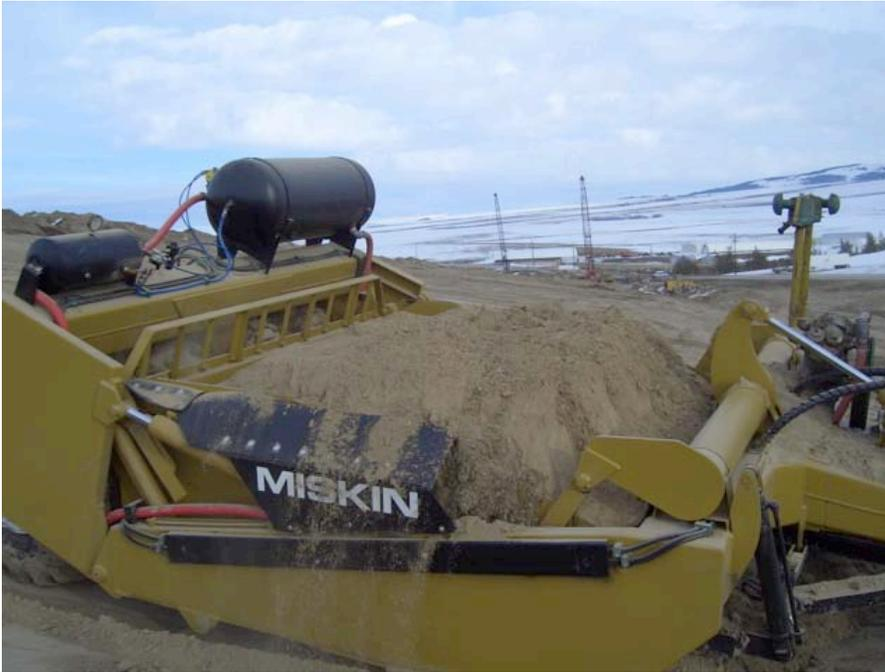
We noticed that the "peak" of an air-assisted load is generally farther forward, than it would be without air. The MisKin "forward reaching" apron will be an important feature on air assisted loads.
