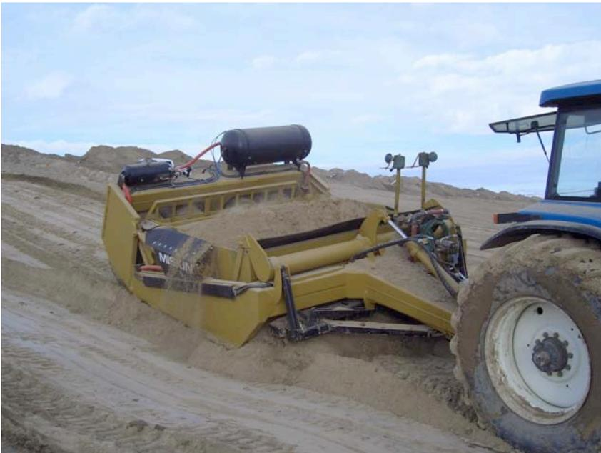
The air changes the dirt in the bowl to a "fluid" state. Note how it is spilling over the sides, without being heaped up. In this "fluid" state, more new dirt can easily enter the bowl.
