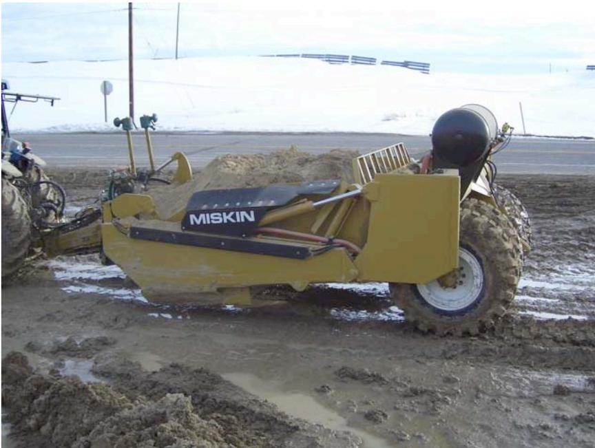
Note how the dirt piles all the way to the top of the Apron Control Pipe (the rest ran off the front and sides).
