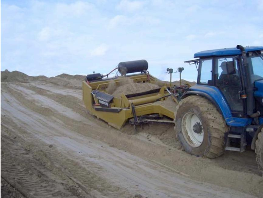
This is about the "most" dust it created at any time. We loaded the scraper as much as we could without the air. Then as the tractor ran out of power, we would turn on the air blast. The tractor lunged forward. From the cab, it felt almost like the scraper came out of the ground (although the digging depth was the same). It was immediately very notably easier to pull, due to the air lowering the scrapers pulling resistance. The tractor immediately gained traction, speed, and momentum.
