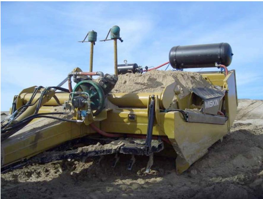
This was loaded with the air assist, in the same distance and time, using the same 142hp tractor. Note that in addition to filling taller, the "corners" of the bowl also filled up much better with the air assist. If the ground had been more moist, the dirt would have stacked up higher.
